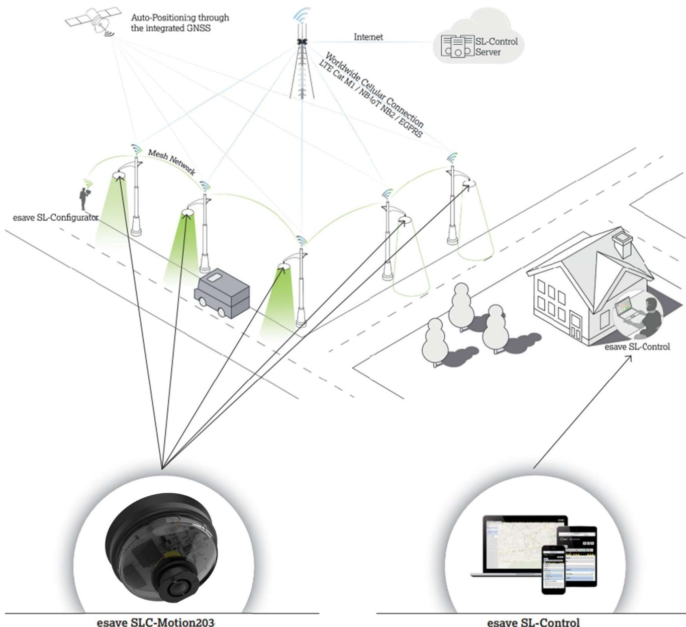
Thanks to the integrated eSIM and gateway function, an SLC-Motion203-C can establish a connection to the SL-Control web platform while maintaining a network with all other esave equipped lights within reach.
