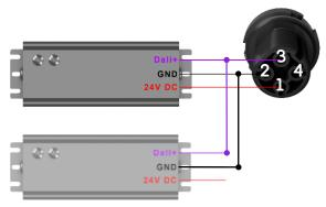
**Note:** The controller supports up to 4 LED Drivers simultaneously.
